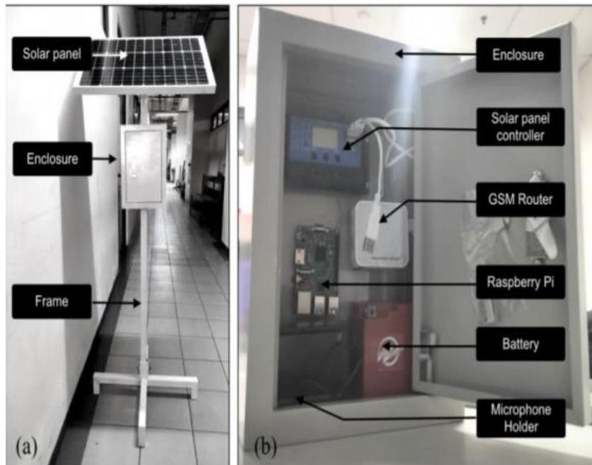
**Figure 1.** The results of the design of a bioacoustic monitoring system (BIAMON)
