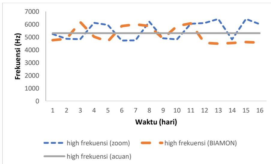
**Figure 6.** Comparison graph of the highest frequency of sound (*Gryllus assimilis*) from the measurement results of BIAMON and ZOOM instruments with reference frequencies
